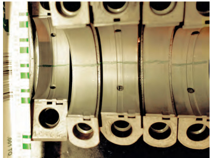
Main bearing shells with Plastigage gap reference
