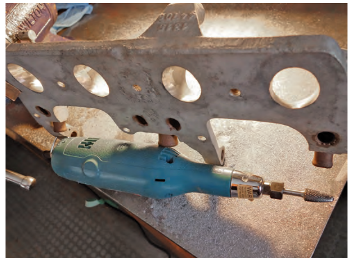
My porting tools for smoothing alignment. Not shown, but important, is my simple dial-in and plug-in speed controller commonly used with wood routers.
