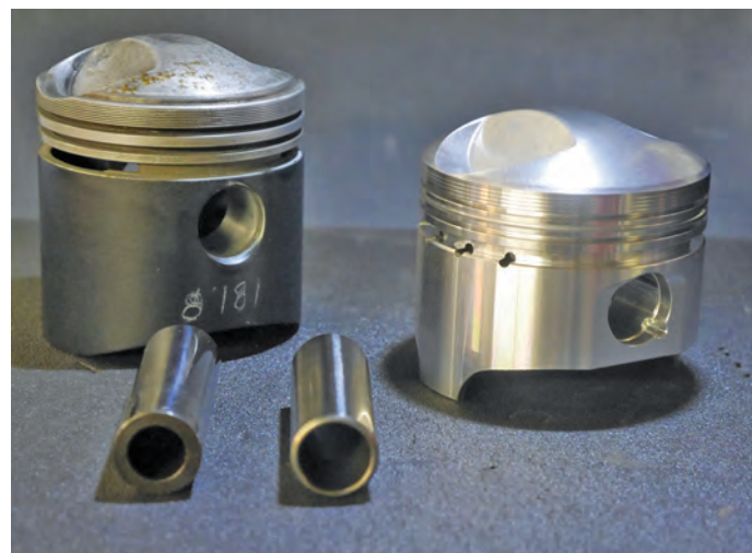
My original plan for increasing torque is on the left but I installed four of the pistons and pins on the right
