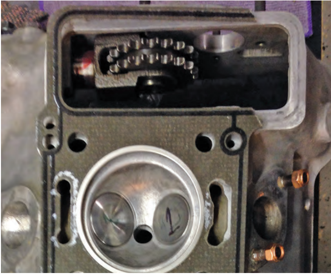
Adapting the best head gasket to fit the 750's shorter chain box is not difficult
